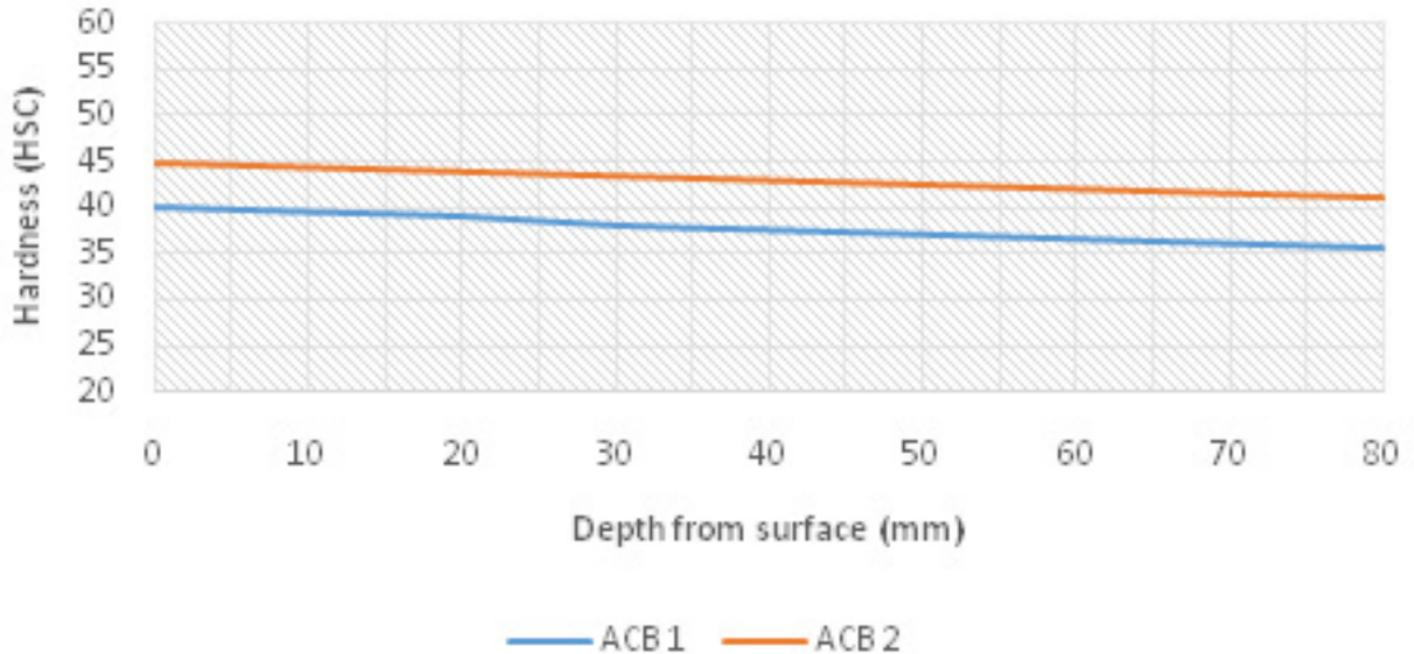
Hardness drop curve for ACB Rolls, ACB: Alloy Cast Steel base
